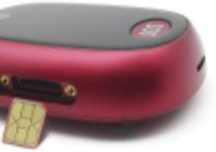
the slot. according to the direction shown in the image. To make the device waterproof, install the SIM slot cover with screws as shown in the image.
