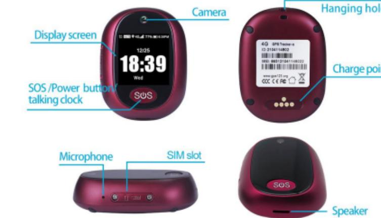
Please use the magnet charger to charge the pendant. Press the power button for 5 to 7 seconds to turn ON. The screen will light up with ringtone.
